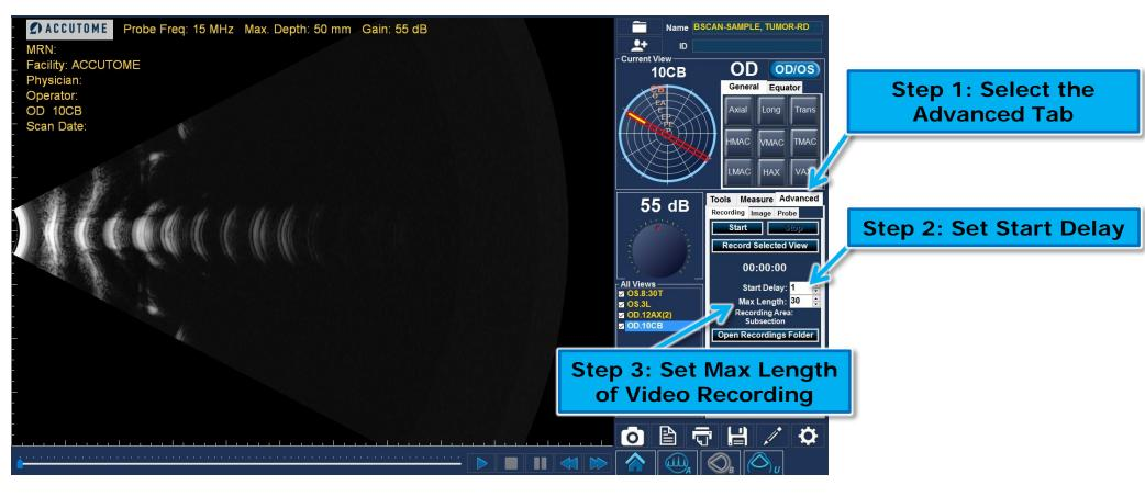
\*Set Start Delay- this delay will allow you to begin recording after a length of time set. It will provide time to get the probe into the correct position before the recording begins.
